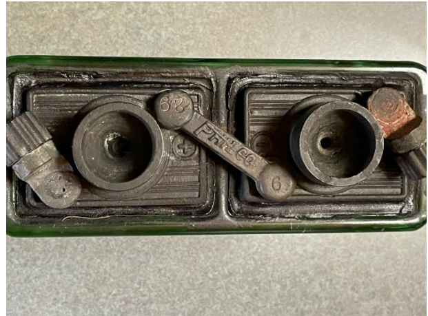
The lid, 42 - 2 , shows PHILCO on the arm connecting the electrodes. Note the two cells are connected in parallel. Courtesy of
