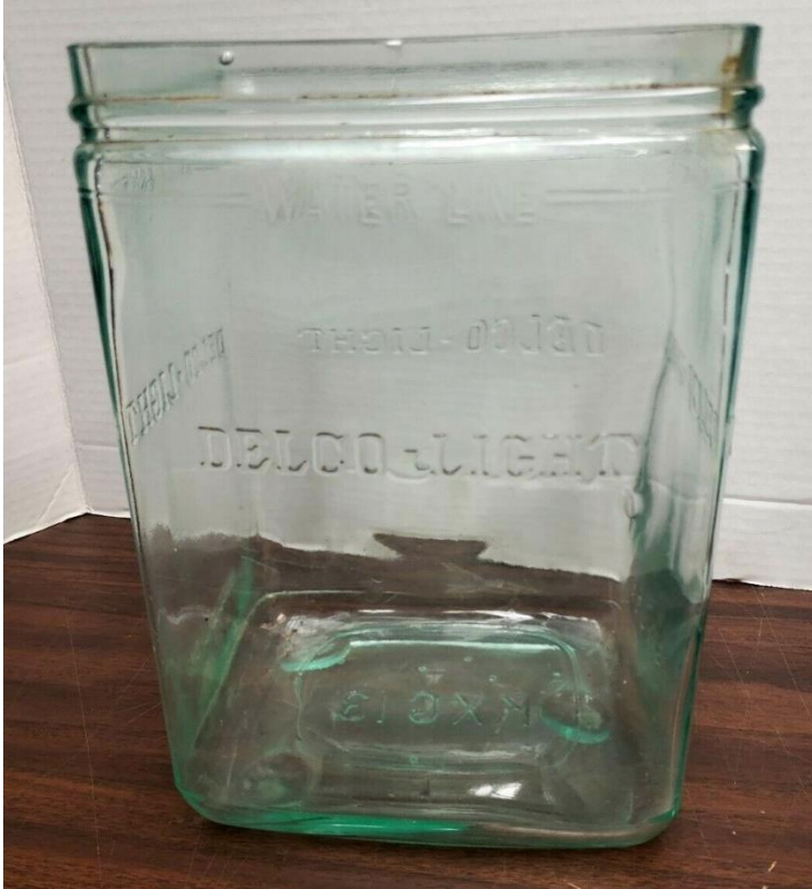
←14 – 3 is aqua with a formed top, Its dimensions are 6”x 7.25” x 10.75” tall. The embossing is WATER LINE / DELCO LIGHT on 4 sides. The botton is embossed KXG 13. Courtesy of mnmama
