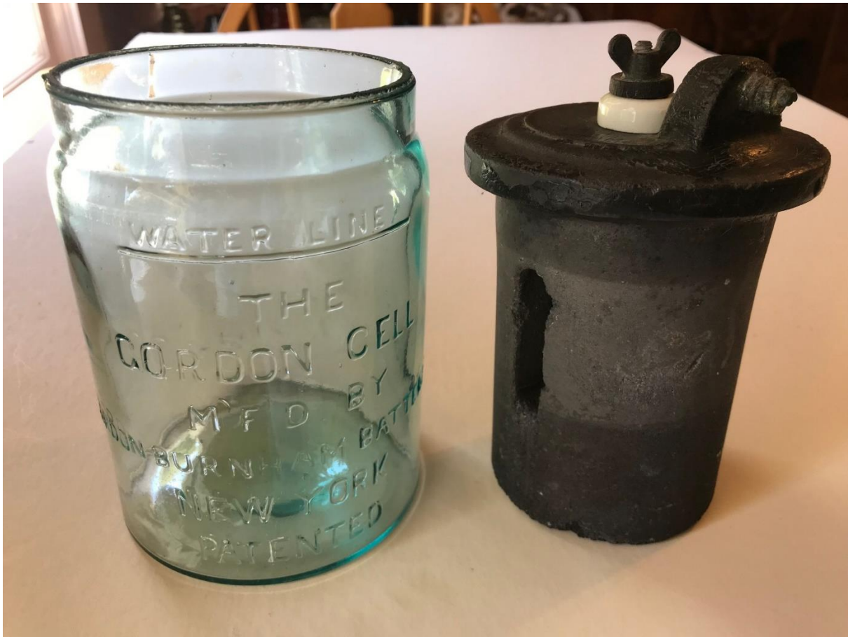
25 - 8↑ is a Gordon cell. It is aqua, with a ground lip, 4.75" diameter x 6" tall with a 4" diameter mouth. It has a combination lid and cylindrical, carbon graphite electrode. It is embossed: Water Line / THE / GORDON CELL / M'FD BY / GORDON _ BURNHAM BATTERY CO./ NEW YORK / PATENTED. Courtesy of Debbi Graham.
