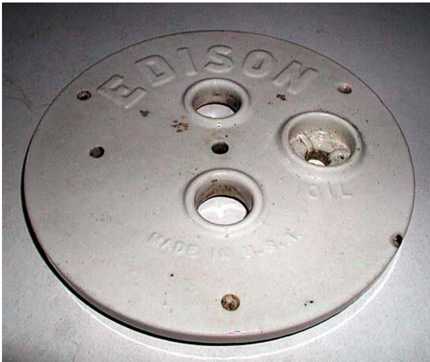
←16 – 7 is yet another embossing variation. It is embossed (arc) EDISON / (arc) MADE IN U.S.A., with a third hole embossed "OIL", for adding battery oil.
