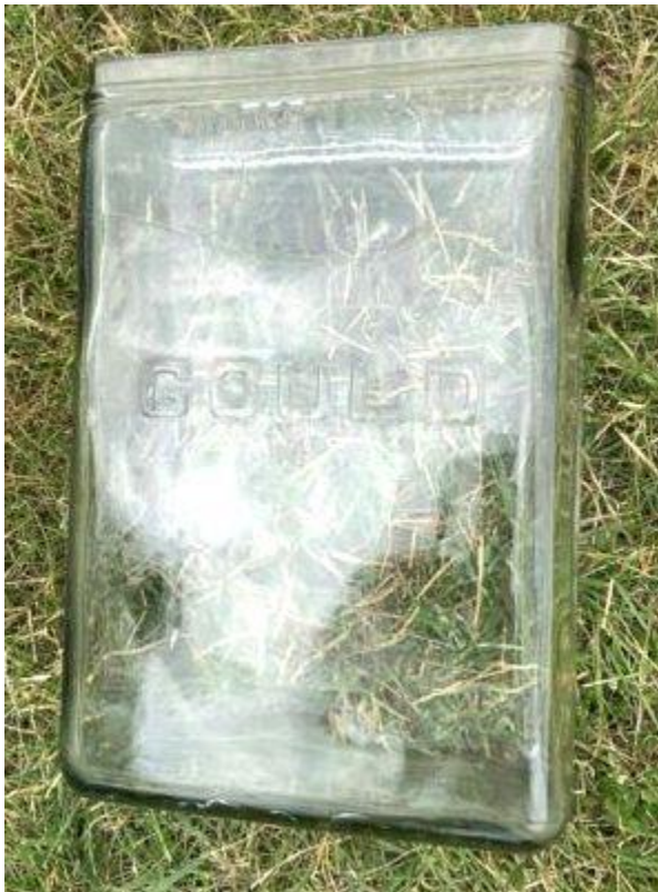
←27 – 4 is a clear glass GOULD battery jar. It has dimensions of 3.75" x 8" x 13" tall. It is embossed WATER LINE / GOULD on two sides.
